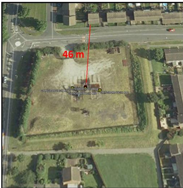
Figure 2: The conventional well Gainsborough 29 (A1) with a setback distance from borehole to the nearest house of 46 m.
